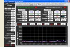
Screen Shot from the Primary DAQ Software Scattering Screen - Monitor and Zero Nephelometers
